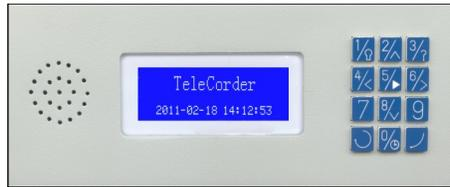
Front panel speaker, LCD display, keypad
